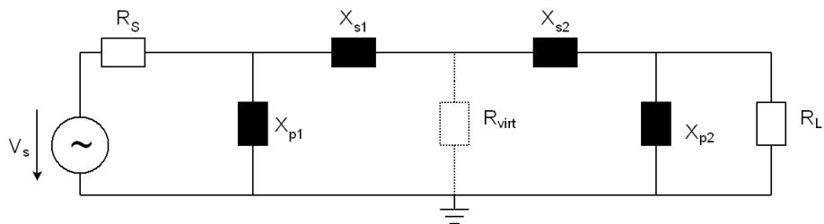
Since  $R_s$  and  $R_L$  make each a shunt circuit, their quality factors are given by :
